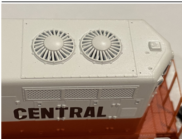
Image 3– The holes are for placing lift rings on the long hood.
