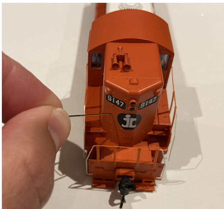
Image 4- The author uses a needle to indent the area prior to drilling to prevent drill bit drift, and reduce the pressure needed.
