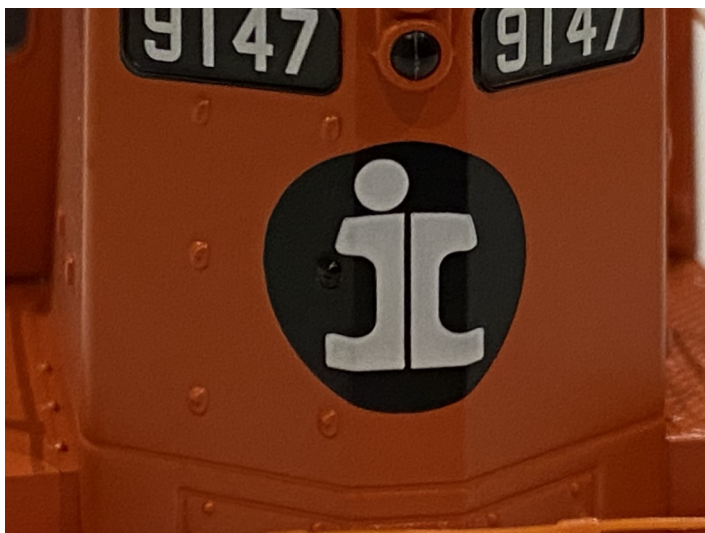
Image 2– The raised bumps are for drilling and placing hand grabs on the short hood.
