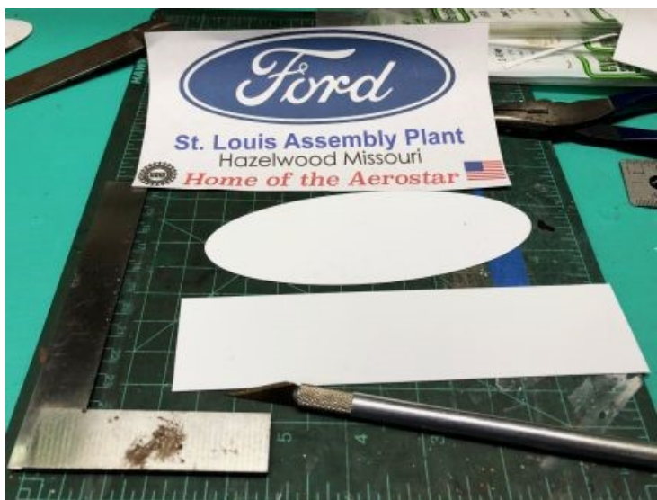
Photo 3- The oval was cut out to the same dimensions as the Ford logo, using a Cricut cutter. The Plant info was a simple rectangle
