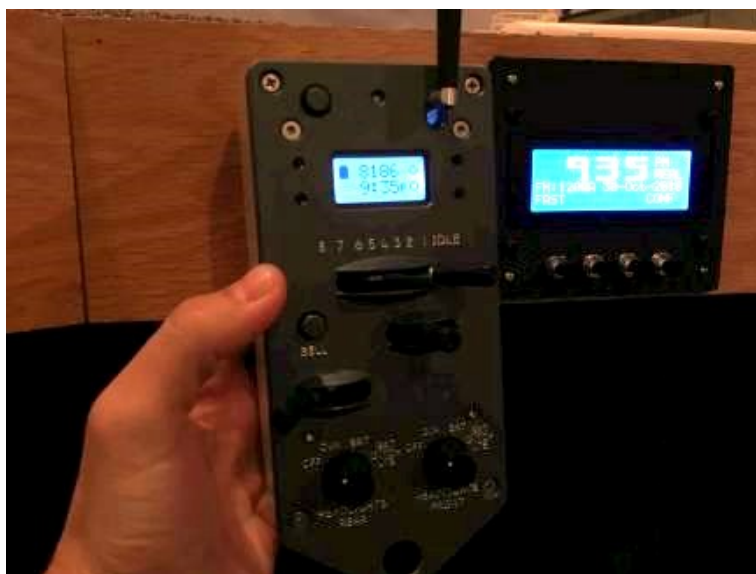
Photo 4: The PT (in hand) can display the fast clock time (right), but you need to have the right components to allow a wireless connection to it.
