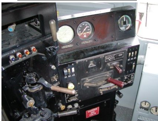
Photo 2: The real "office" of an EMD GP38-2 locomotive, and you can see the similarities to the ProtoThrottle. (Joe Atkinson photo)
