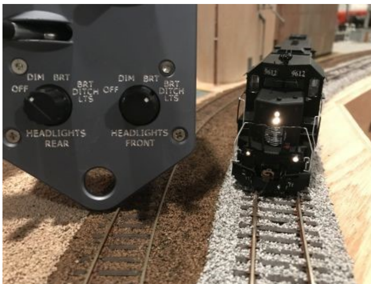
Photo 3: The ProtoThrottle has easy to use light controls along the bottom edge for implementing prototype light control.
