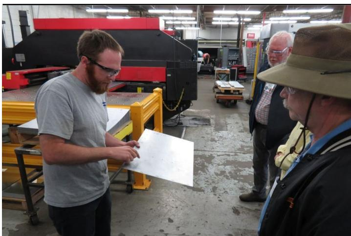
*The tour guide explains how the stamping machine in the background punches out the metal in different shapes and patterns for assembly.*
