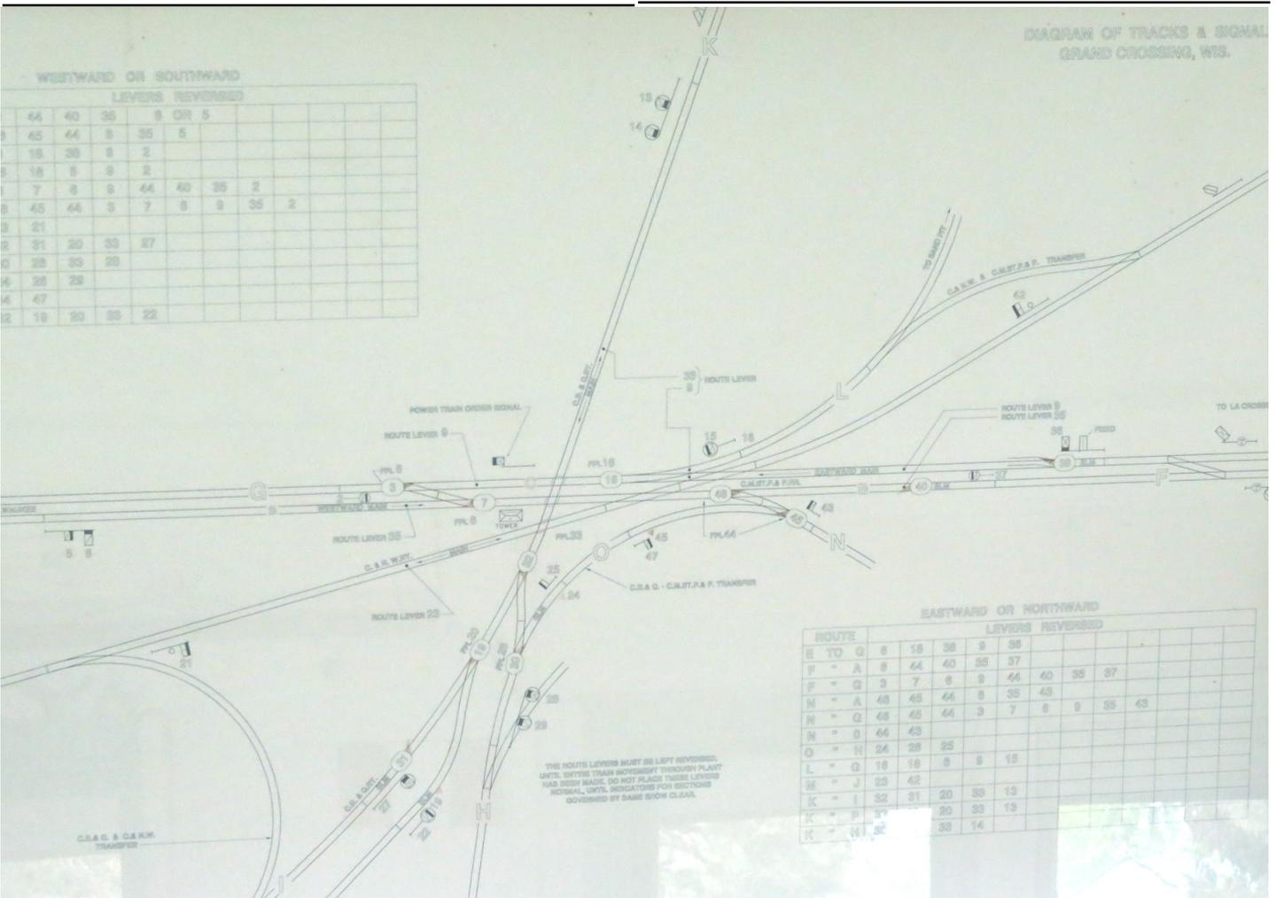
The Grand Crossing tower controlled the diamonds between the CB&Q single main from the north, the CNW from the Northeast diagonally to southwest, and Milwaukee's double main from the east. There are numerous interchange tracks connecting the mainlines.
