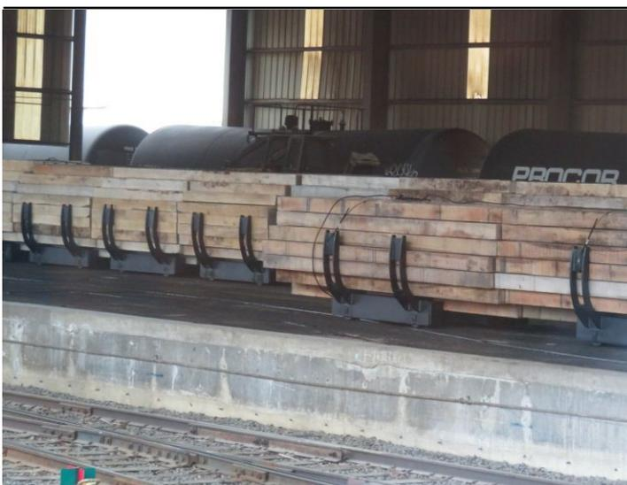
*Dry ties are stacked on dollies prior to being pushed into the massive retort that will use high pressure to force creosote into the wood.*
